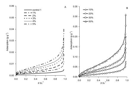
Fig. 1. Water vapour adsorption isotherms for mixtures of podzolic soil formed from loamy sand with organic fertiliser Rosahumus. Part A – dose of Rosahumus from 1 to 5%. Part B – dose of Rosahumus from 10 to 50%
