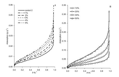
Fig. 2. Water vapour adsorption isotherms for mixtures of podzolic soil formed from loess with organic fertiliser Rosahumus. Part A – dose of Rosahumus from 1 to 5%. Part B – dose of Rosahumus from 10 to 50%
